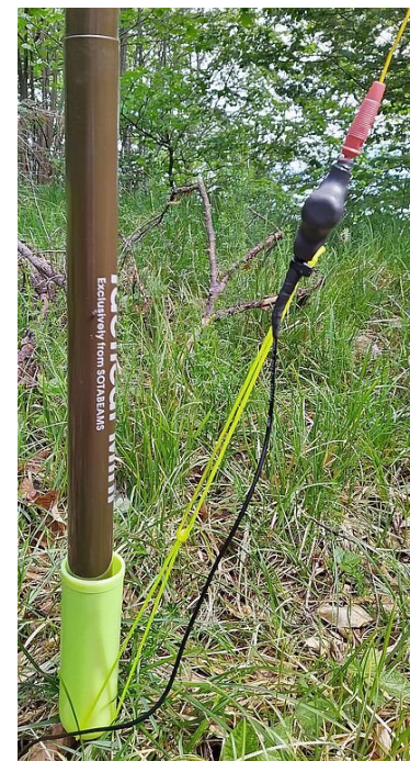
Figure 45: Holding the coupler in place with a cord
