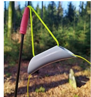
Figure 5: Top radiator wire support
