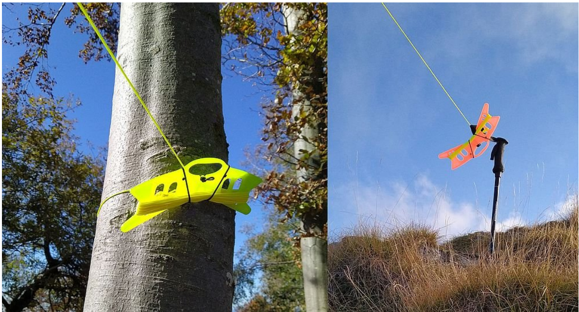
Figure 44: Quickly attaching the antenna cord with the wire winder
