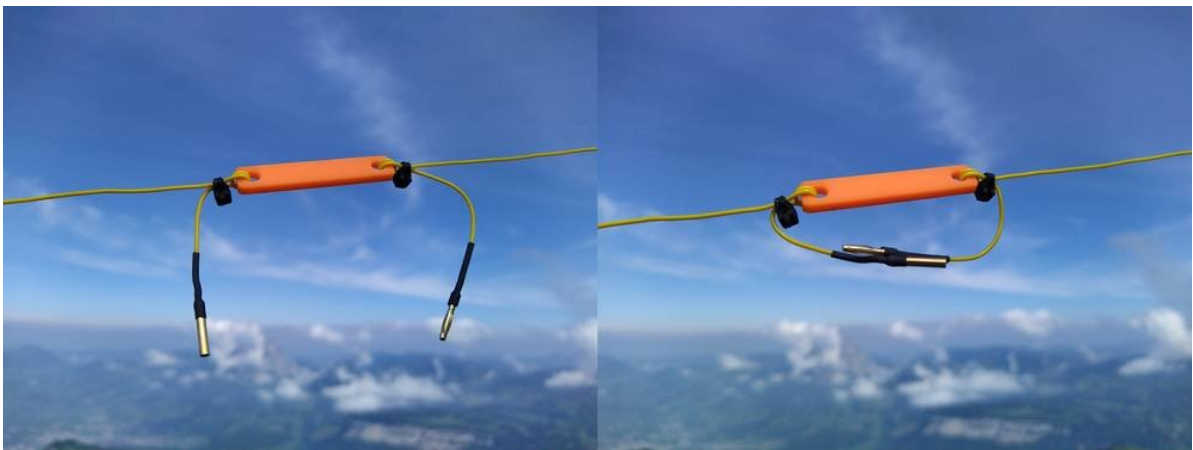
Figure 43: Open link comparison: 200kHz resonance difference at 18MHz
