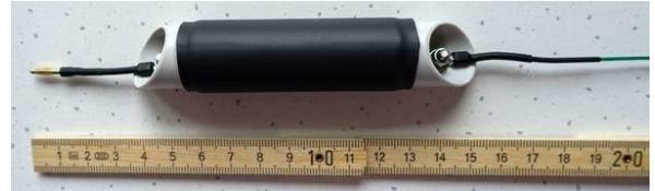
Figure 32: Finished 80-meter-band loading coil with 2mm gold plated plug
