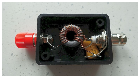
Figure 13: A compact coupler as backup
