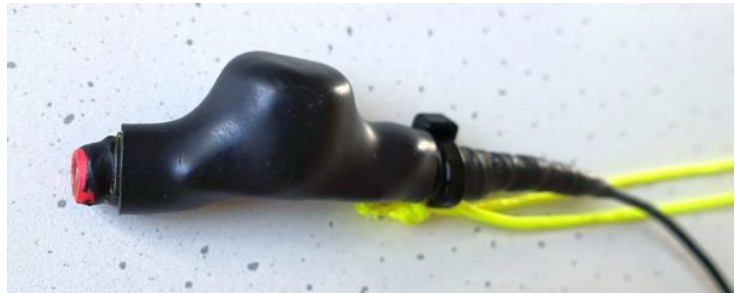
Figure 25: 1:64 coupler after more than 150 SOTA activations
