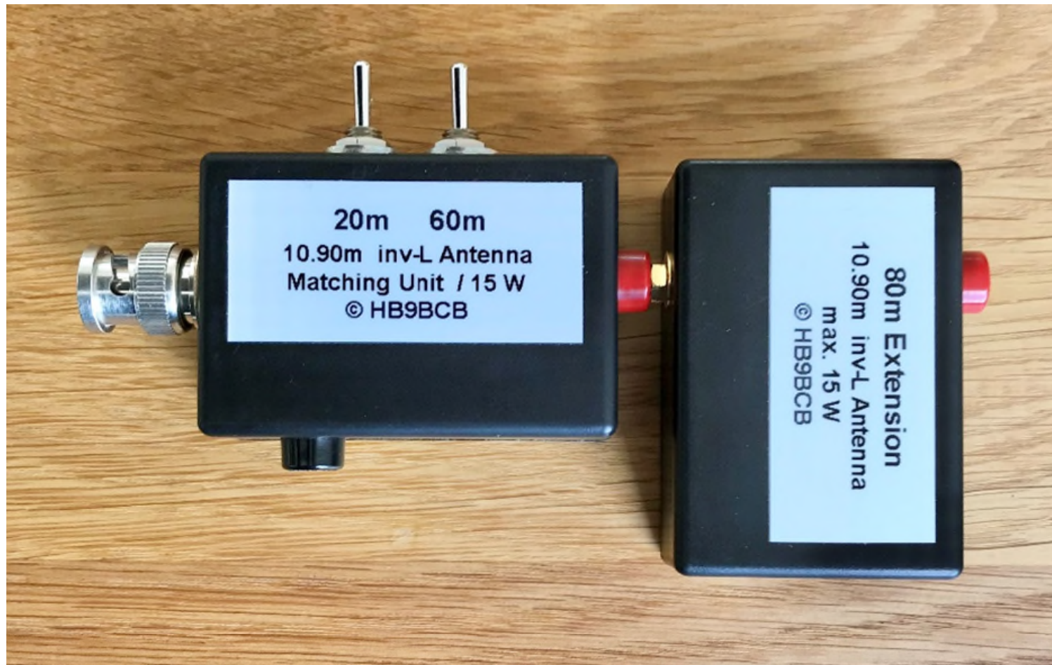
Figure 11 External impedance matching aids for 20, 60 and 80 m
