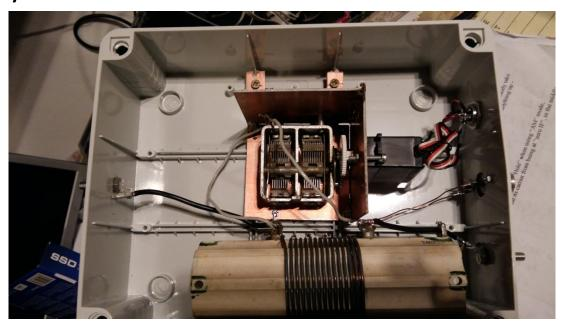
Servo motor (controlled from the shack by a small AVR microcontroller) drives a variable capacitor for optimal antenna resonance.
