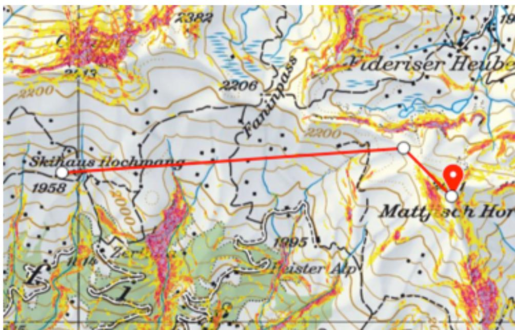
*The red/yellow areas indicate slopes >30 degrees (the critical angle for avalanches). As you can see, the route to the summit is virtually clear of any such slopes.*
