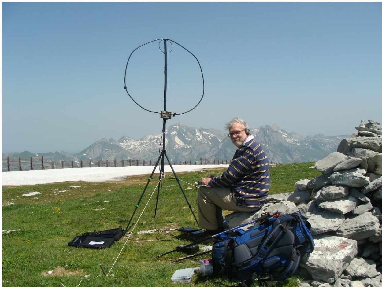
My operating position at a cairn with my AlexLoop. It was very windy that day and I had to use cord to stabilize my antenna. You seldom see an activation zone so large at this altitude. You can use the posts on the snow fence for a mast support, but even in late June this would involve getting your feet wet.
